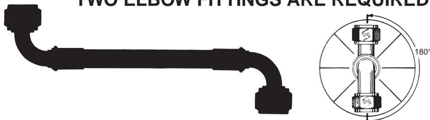
**MEASURING:** When installations require hose assemblies with elbow fittings on both ends, hold the assembly so that the nearest fitting is pointing in the 6 o'clock position. Measure angle between fittings, counterclockwise. Both fittings pointing to 6 o'clock will be specified as zero degrees (0°)
